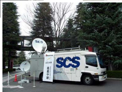
Satellite Relaying System
