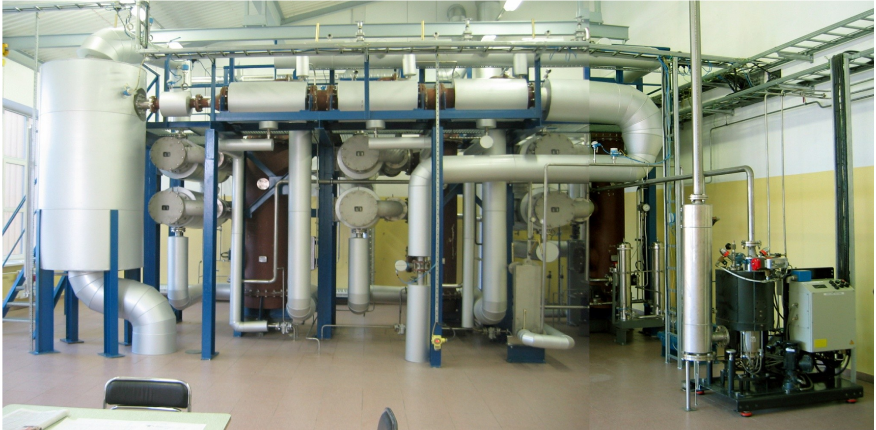
Beverage alcoholic manufacturing Plant in Europe (1250kg/h of ethanol)
