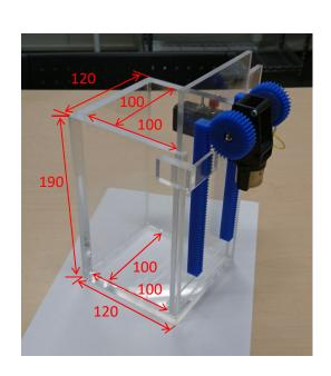
Thickness of side acrylic boards: 10mm
