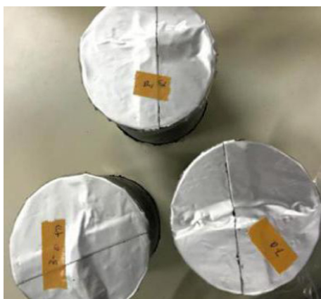
Fig. 2. Specimen's section sealed with waterproof tape.
