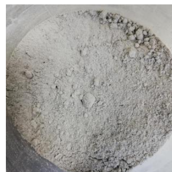
Fig. 1 Municipal solid waste incineration fly ash (MSWI-FA).
