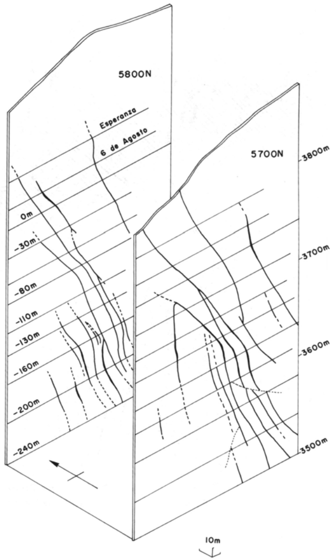
FIGURE 31. PANEL DIAGRAM SHOWING VEIN PATTERN IN THE DON PEPE SECTION, CARACOTA MINE.
