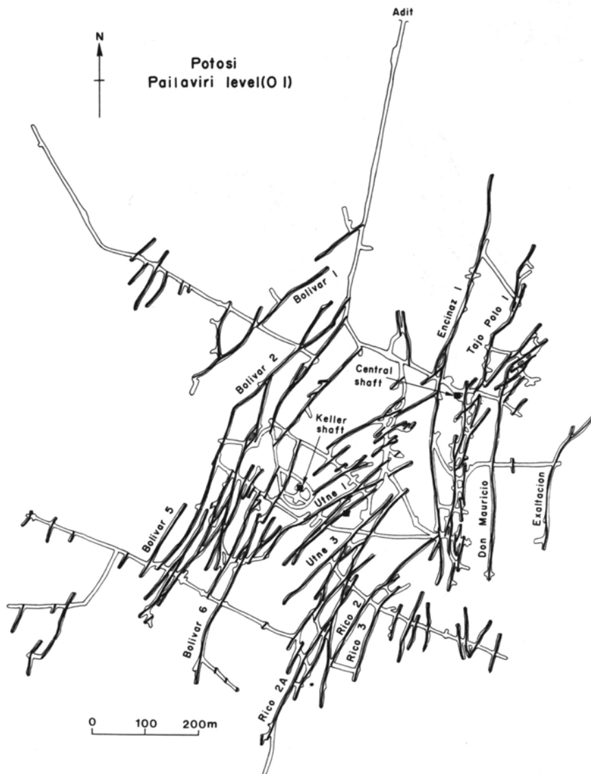
FIGURE 19. VEIN ARRANGEMENT AT THE 0 (PAILAVIRI) LEVEL, POTOSI MINE.
