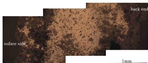
Figure 7. Photomicrograph of ore microscope under reflected light for cross section of sample No. 1. (Light brown: copper rich metal phase, dark brown: secondary product.
