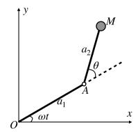
$\dot{x} = -\alpha_1 \omega \sin \omega t - \alpha_2(\omega + \dot{\theta}) \sin(\omega t + \dot{\theta})$   $\dot{y} = \alpha_1 \omega \cos \omega t + \alpha_2(\omega + \dot{\theta}) \cos(\omega t + \dot{\theta})$
